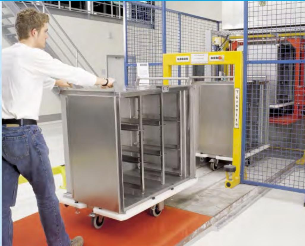
The HUPFER® container and sterile goods trolley has been developed especially for automatic guided vehicle systems (AGV) - it is shown here in the automatic run-in to a multi-chamber washing installation.
