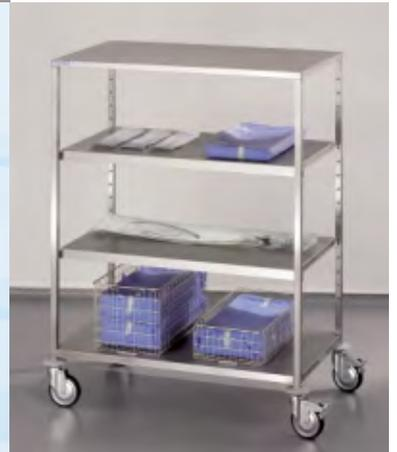
The chassis consists of 4 steering castors, of which 2 can be braked, with double-ball bearing, in galvanised-chromated casings, Ø 125 mm. The castor material is antistatic. Further designs, such as for example castors which are suitable for trolley washers and which can be sterilised are available on request. Wall protectors in abrasion-resistant plastic effectively protect the trolleys from damage during transportation.
