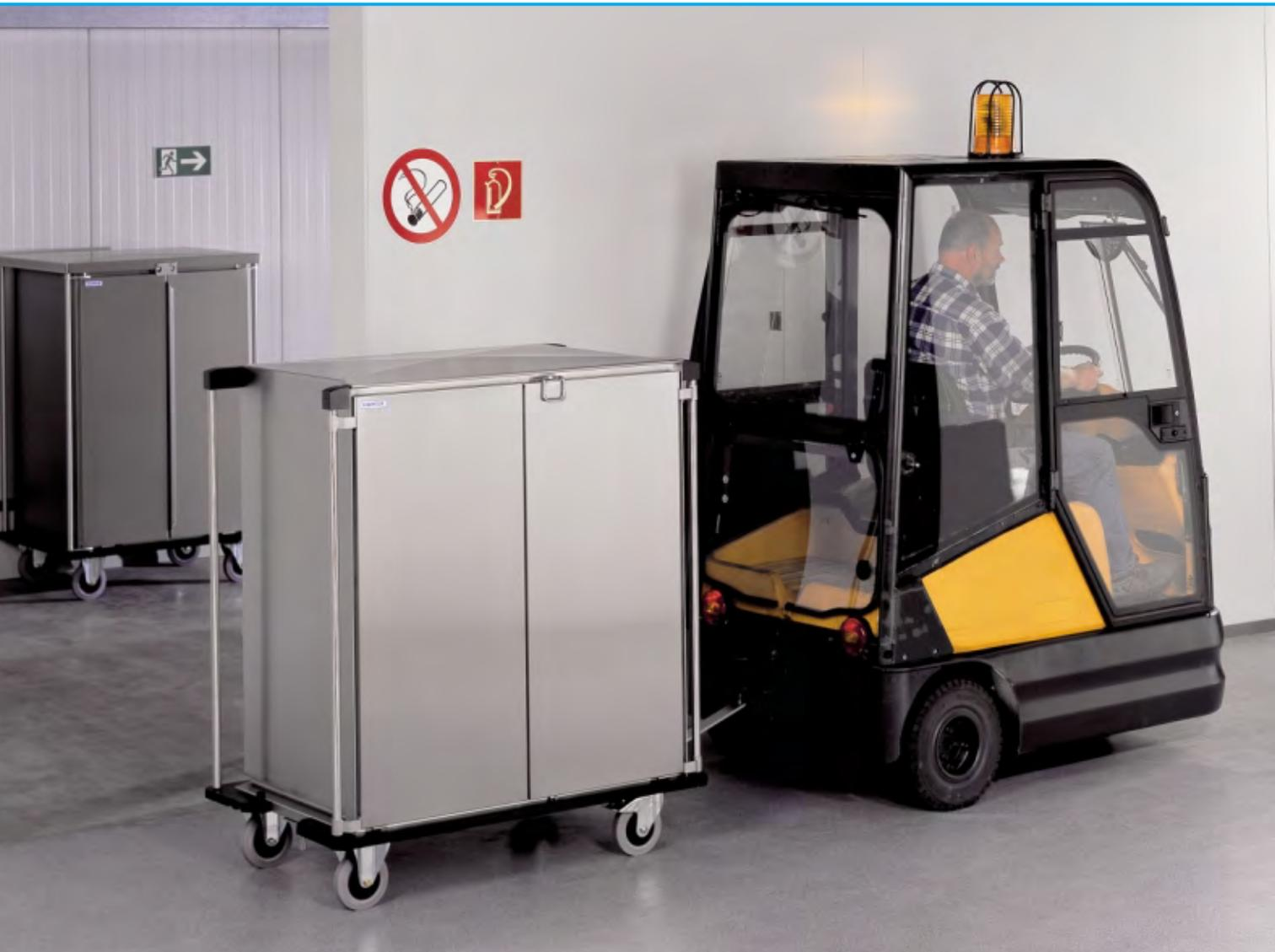
All HUPFER® closed container and sterile goods trolleys can be equipped with a coupling and a towing bar. A friction-damped coupling is available for towing several trolleys without any rolling motion. Castors of an excellent quality and an impact-resistant protective bumper effectively ensure safe transportation.
