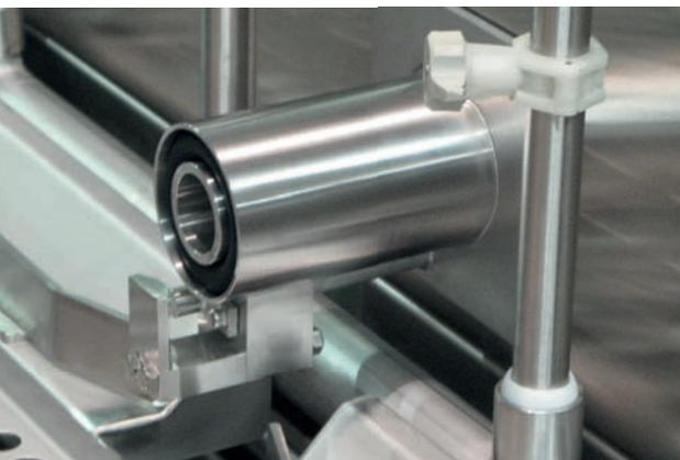
*The patented connection coupling with special sealing mechanism ensures constant-pressure, leakage-free supply to the cleaning system and consequently a better cleaning result with higher washing nozzle pressure.*
